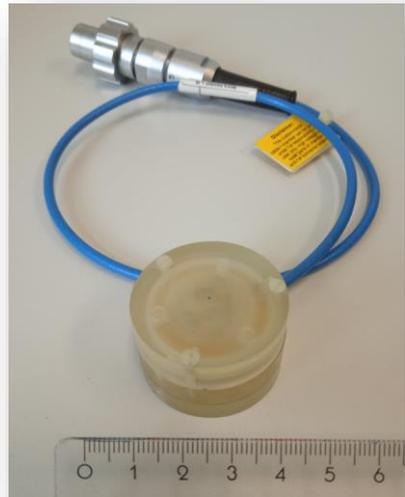
**Fig. Ionization chamber prototype (0.27 mm)**
