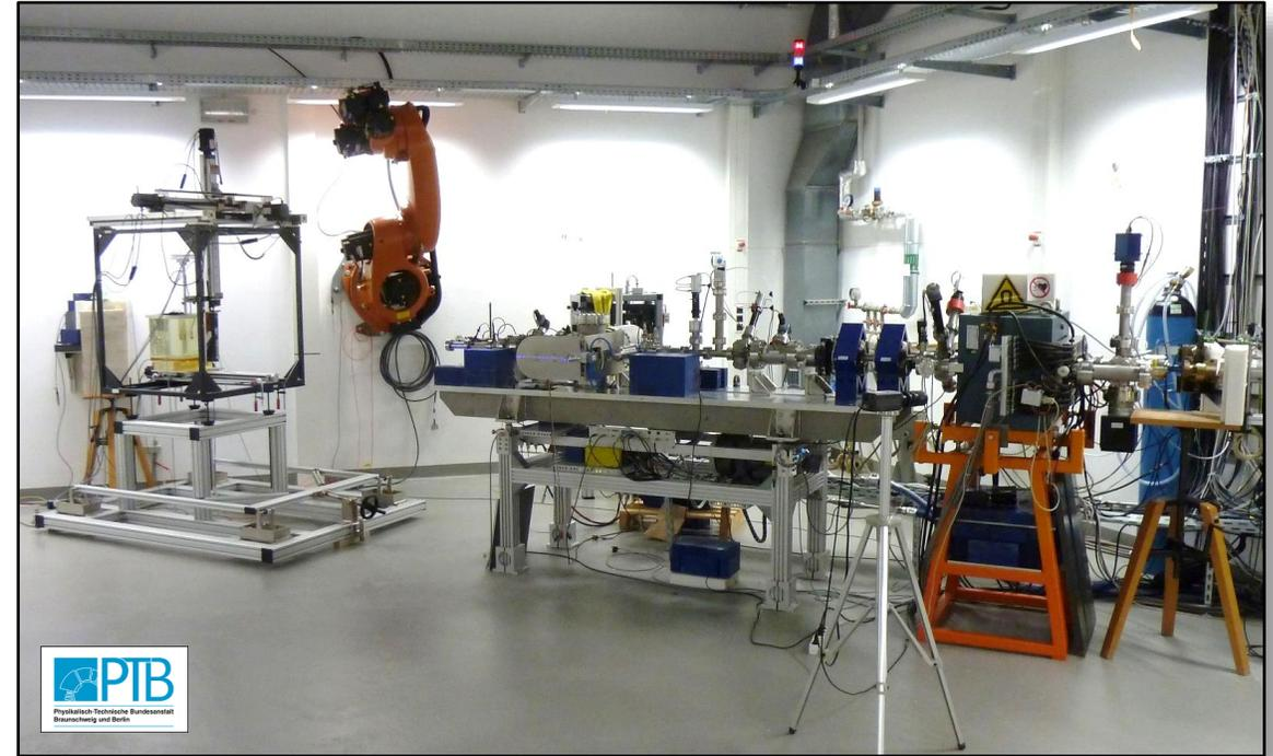
*Beam line with water phantom*
