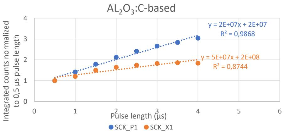
Ok linearity with pulse length (dose per pulse), low saturation observable
