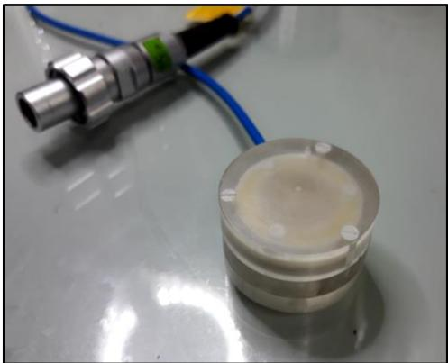
*Ionization chamber prototype (0.27 mm)*
