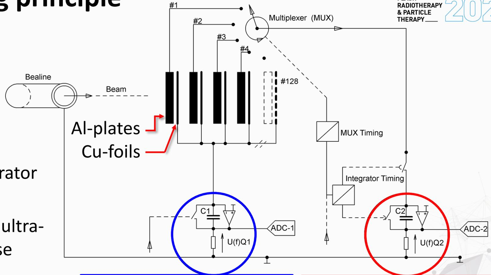
Current-Integrator #1: monitoring of the total image charge on Cu-foils
