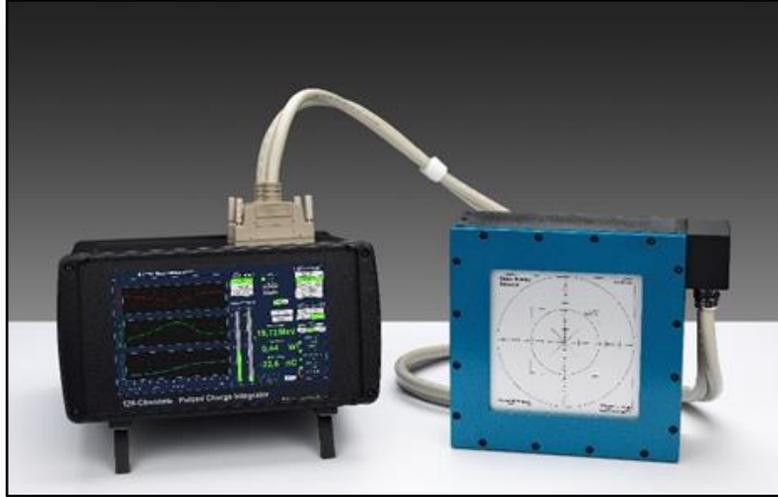
PTB developed a portable Multi-leaf Faraday Cup (MLFC) for energy determination of charged particle beams
