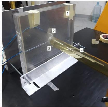
1 PMMA Phantom
