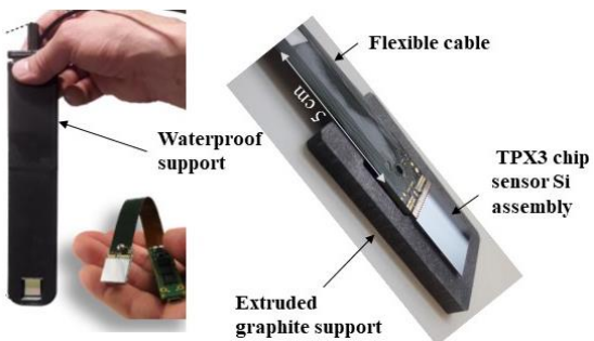
Figure 1. Customized MiniPix TimePix3 with the electronic design located at 5 cm distance from the active surface. All metal holders, screws and cooling elements were changed with carbon or ABS plastic.
