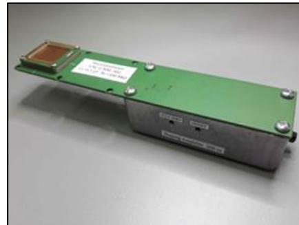
*Microdosimeter with electronics assembly from USC*
