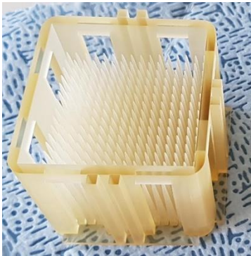
3D-printed range modulator
