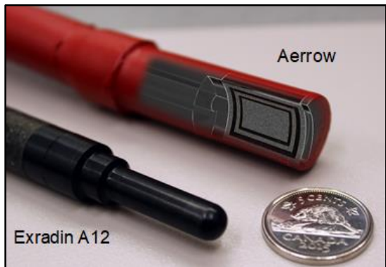
Calorimeter Aerrow (and ionization chamber)
