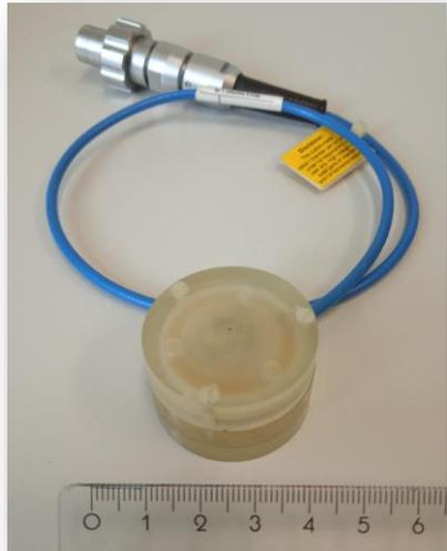
**Fig. Ionization chamber prototype (0.27 mm)**
