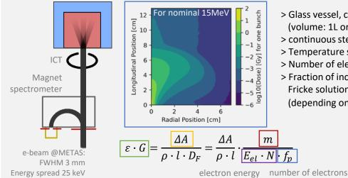
> Glass vessel, closed using a 50µm polyethylene foil (volume: 1L or 2L)
