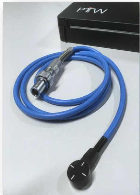
Fig. PTW IC prototype (0.25 mm)
