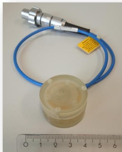
Fig. Ionization chamber prototype (0.27 mm)
