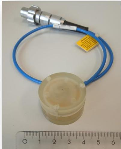
Fig. Ionization chamber prototype (0.27 mm)
