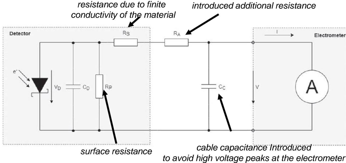
**Fig. Circuit representing microDiamond detector (equivalent to diode)**
