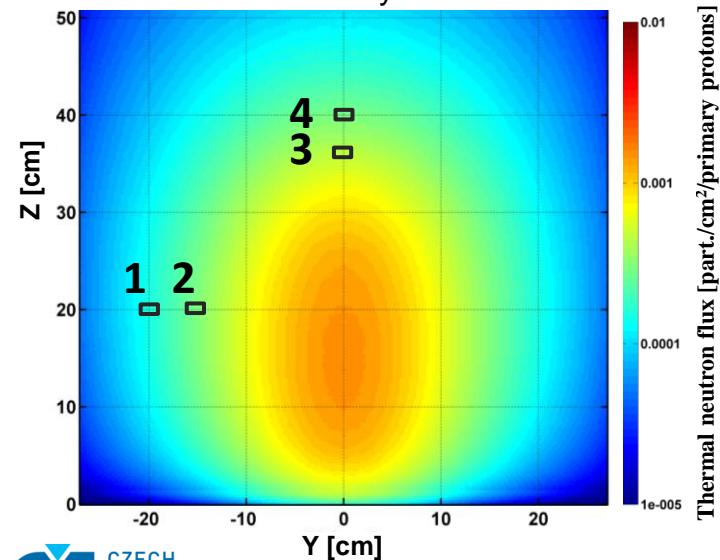
*Measured thermal neutron flux for a DR at the reference point of 0.27 Gy/s*
