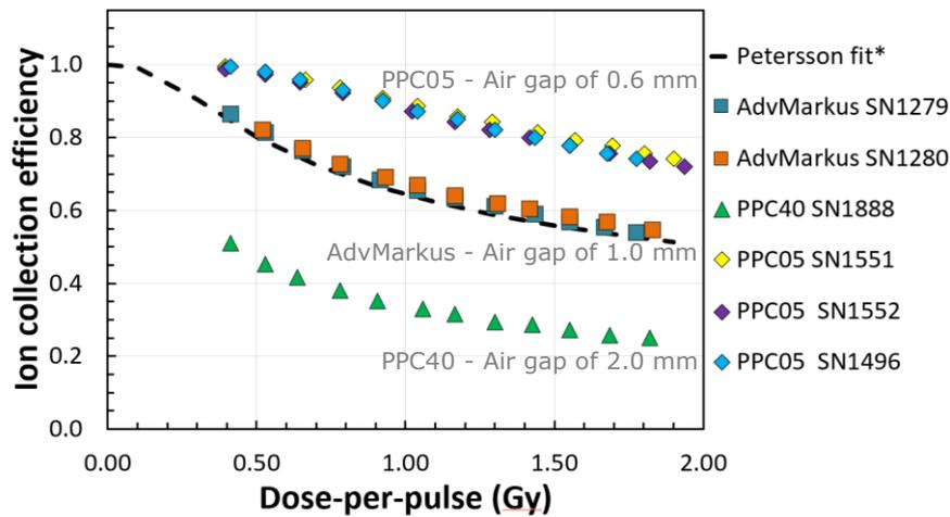
**Figure 3:** Ion collection efficiency in ultra-high dose per pulse electron beams
