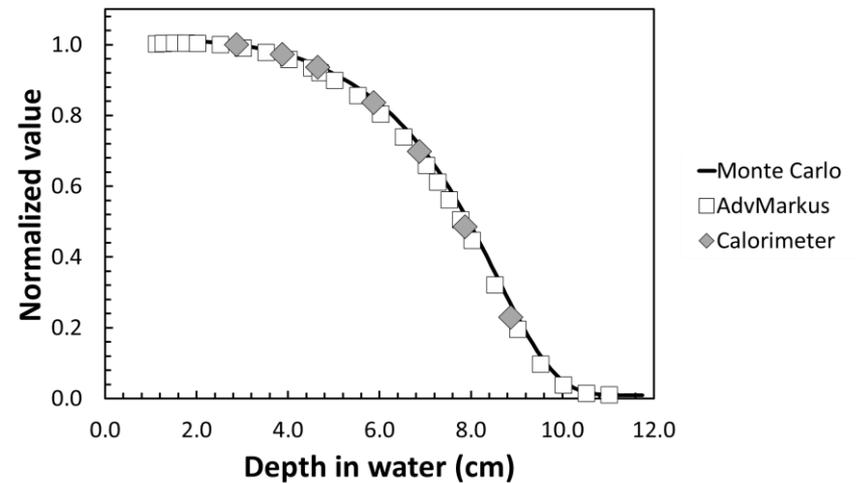
**Figure 4:** Depth dose measurement in water with calorimetry and ionometry compared to Monte Carlo simulation.
