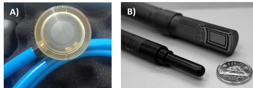
**Figure 2:** A) Picture of an Advanced Markus ion chamber. B) Picture of the Aarrow (top) with a cross-sectional drawing compared to an Exradin A12 (bottom left) ion chamber and a 5-cent Canadian coin (21 mm wide).
