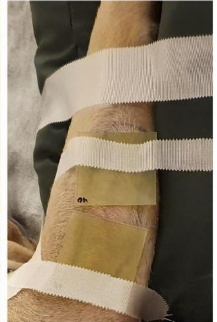
*treatment of the leg with in vivo dose measurements by radiochromic film*
