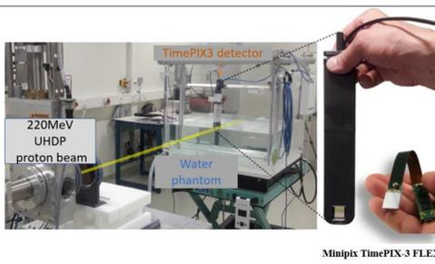
Figure 1. Experimental setup at the University Proton Therapy Dresden, with Minipix-Timepix3-Flex detector placed in a waterproof cage. The detector chip-sensor assembly (shown on the bottom right) is detached from the readout electronics board.
