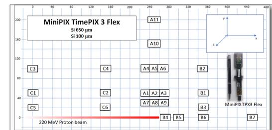
Figure 2. Experimental setup at the University Proton Therapy Dresden with identification of the positions where the detector was placed inside the water-phantom.
