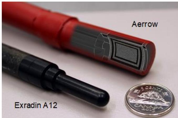
*Aerrow (and Exradin A12 ionization chamber for size reference). The internal structure of Aerrow is shown as a blended rendering.*
