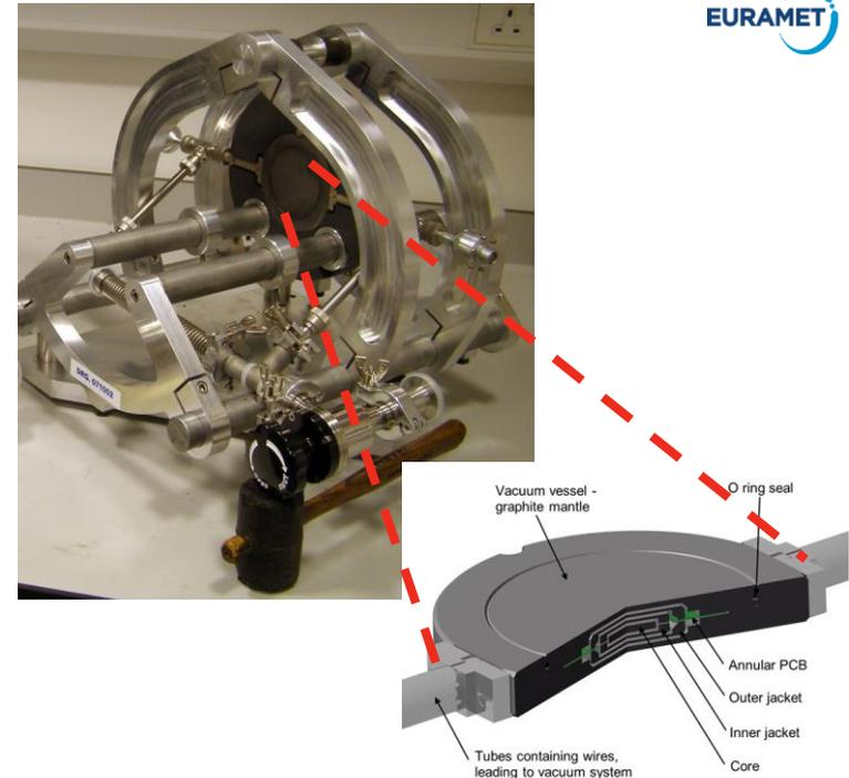
**Fig. 1:** NPL's primary standard graphite calorimeter.
