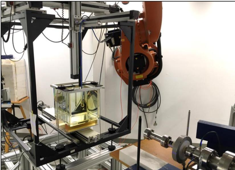
*Detector under test at reference depth
