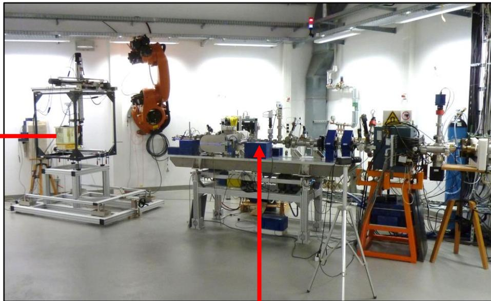
Non-destructive absolute beam pulse charge measurement (uncertainty < 0.1 % @70 nC/pulse)
