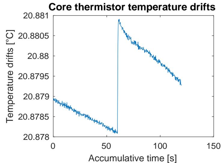
Radiation induced temperature rises of one of the core thermistors for first laser shot
