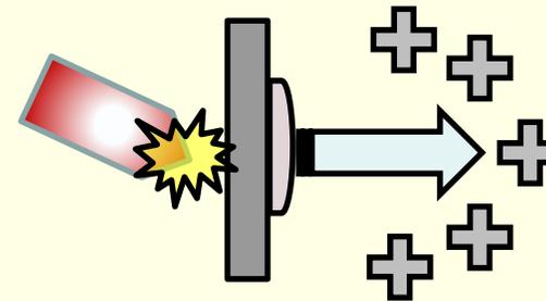
Protons produced through laser-target interaction (TNSA mechanism)
